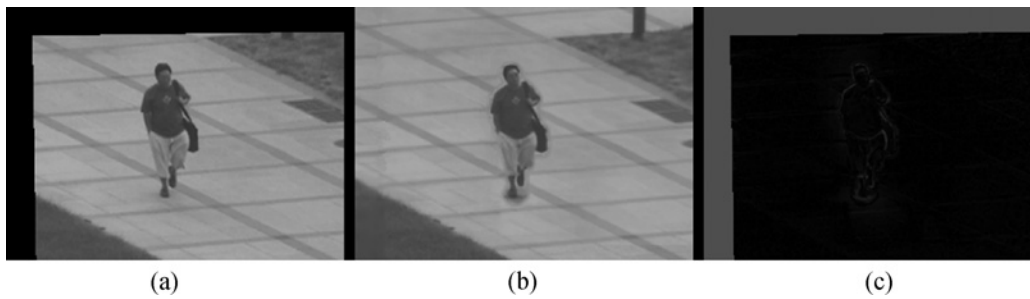
Fig. 11. Testing of high-resolution inpainting. (a) Ground truth. (b) Inpainting result by assuming that M_{LH}^t is invalid. (c) Absolute difference between (a) and (b).
